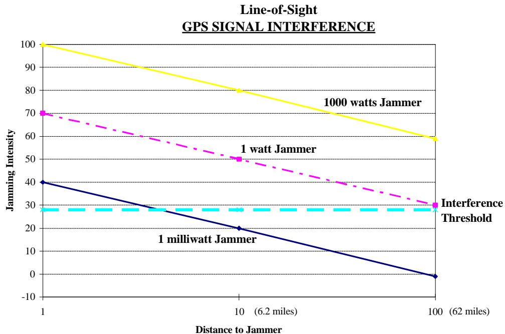
The horizontal axis represents the distance between the jammer and the typical Global Positioning System receiver in kilometers. The vertical axis represents the jammer interference to the Global Positioning System signal in decibels (dB) or the jamming intensity. The three diagonal parallel lines represent three jamming devices with different effective power measured in watts and milliwatts.
