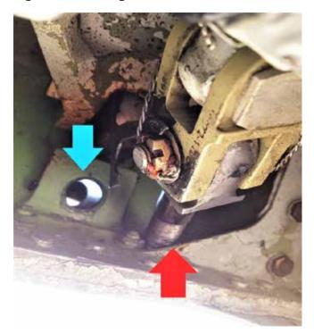
The photo shows an MD-80 elevator rod (red arrow) dislodged from its mounting hole (blue arrow) because it was not properly secured with a cotter pin (not shown).
