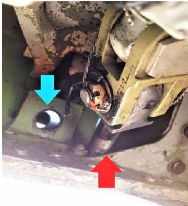
The photo shows an MD-80 elevator rod (red arrow) dislodged from its mounting hole (blue arrow) because it was not properly secured with a cotter pin (not shown).
