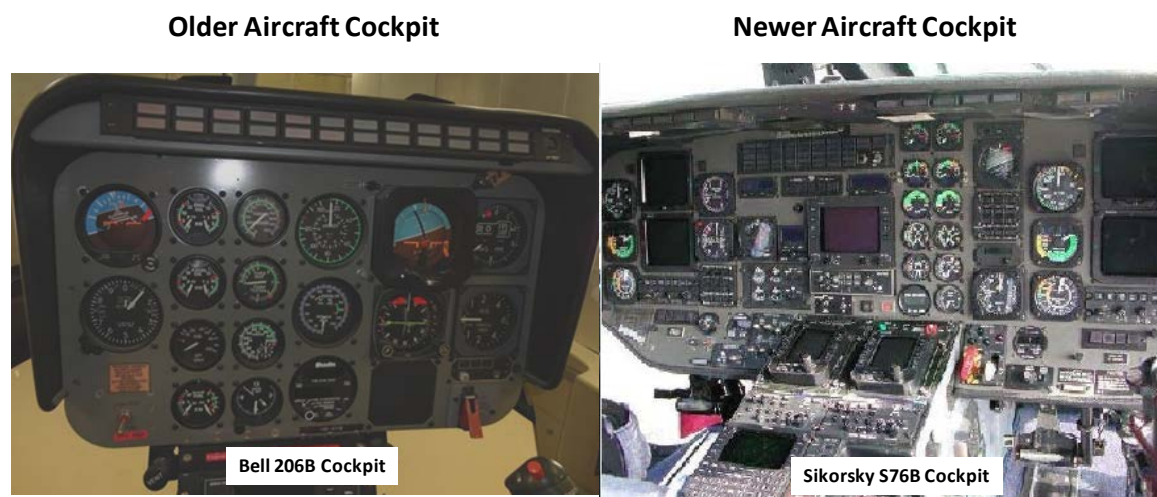
Figure 6. Helicopter Cockpit Complexity Comparison
